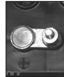
POSITIVE POST HAS LARGER DIAMETER
