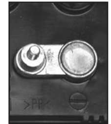
NEGATIVE POST HAS SMALLER DIAMETER
