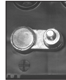
POSITIVE POST HAS LARGER DIAMETER
