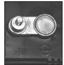
NEGATIVE POST HAS SMALLER DIAMETER
