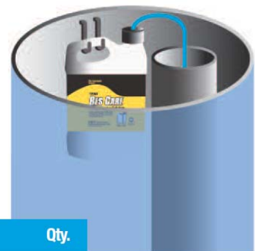
A. Pro Easy Feeder mounts the 64 oz. Res Care® feeder bottle on inside wall of Brine Tank B. Wick is suspended inside brine well to facilitate automatic dispensing
