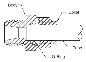
Figure 2 - Quick Connect Fitting
