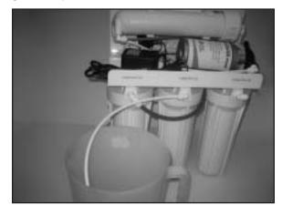
Figure 10 - Direct flushed water and carbon fines into container
