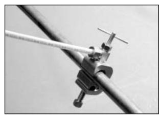
Figure 3a Feed Water Assembly
