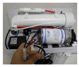
19. Connect one blue wire and two black wires using the blue wire nut provided. Connect the other blue wire and two black wirers using the other blue wire nut provided.
