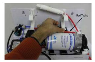
15. Take the white tubing collected from step 4. Connect the tubing (the end without the nut) to the high pressure switch. Install the RO Membrane housing back to it clips and re-connect the other end of the white tubing to the membrane housing.
