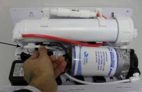
3. Remove the RO membrane housing from the clips and hang it to the side of the RO Module
