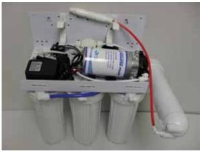
4. Remove the white tubing from the Auto Shut off as shown below. This tubing is the other end of the tubing removed from the RO membrane housing. Pull this white tubing out from the RO bracket/module and save it for future use for this installation.
