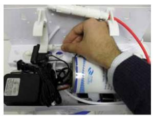
7. Remove the white tubing connection to the outlet of the booster pump.
