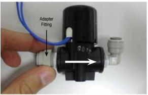
9. Attach solenoid valve to the bracket with the screw provided. Please refer to the pictures below.
