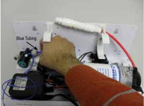
12. Connect the 19" black tubing to the inlet of the booster pump and connect the other end to the outlet of the solenoid as shown below.
