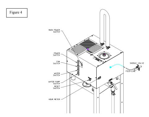
3. Your distiller has been shipped with a sterilization drip tube that is to be placed between the cooling coil and the storage tank. The tube end should be inserted into the storage tank properly. As your distiller continues to heat up, you can sterilize your distiller by simply turning the fan switch off for approximately ½ to 1 hour. Leaving the storage tank lid on. After this cycle is completed, turn the fan switch on and drain any excess water from the storage tank.
