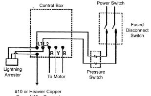
Ground Wire Connect to 8 ft. Ground Rod or Well Casing
