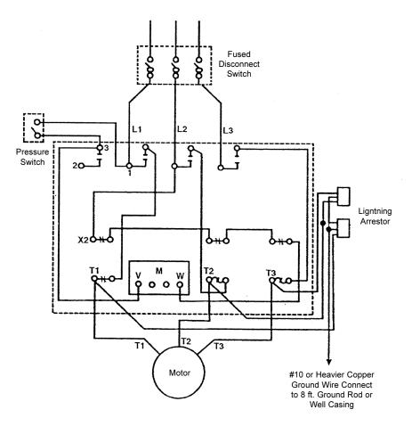
WARNING: Connect motor leads momentarily for correct rotation before installing pump in well.
