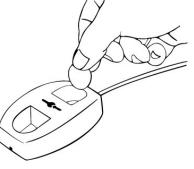
The controller should be tested every month, at both the controller and sensor(s) to confirm the system operation and to exercise the valve.
